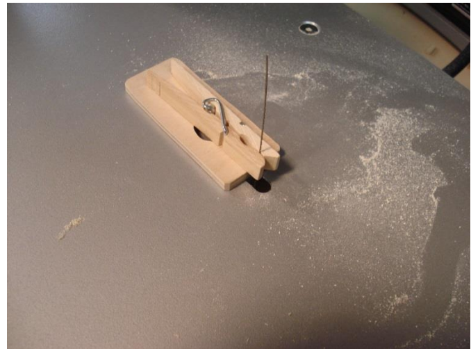
H. You can now put both hands under the table to secure the blade
