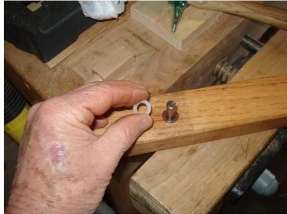
One other place I checked to eliminate the noise was the drive arm of the eccentric drive shaft. It had a plastic bushing sleeve in it, and it was worn in an oblong shape. I was able to purchase a new one and that eliminated about 90% of the noise.
