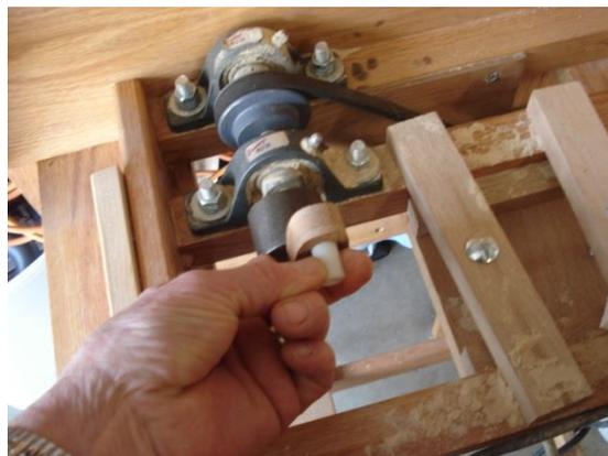
I put it all back together, with grease in the bronze bearings, and squared the blade up by shimming one side of the table, up about 1/16". It runs much better, but the bottom blade clamp is a **big headache** to adjust or change the blade. This saw is much more for 'atmosphere' in my Branson shop, not for easy and accurate cutting. I have been spoiled by my Excalibur saw's accuracy and ease of use.
