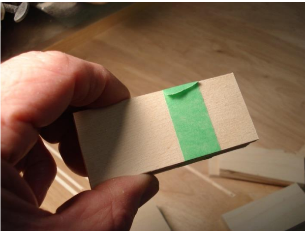
A. Tape up (3) 1- 3/8" X 3 -1/8" X 1/8" BB plywood
