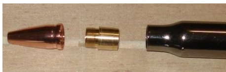
Tip unscrewed from insert-(ready to be glued into the pen's end)
