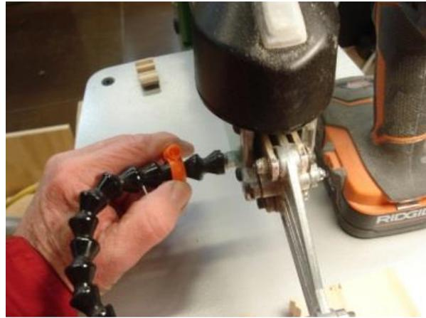
Place the clamp over the tip, and slide it up in place over the loose link. Install the screw and tighten.
